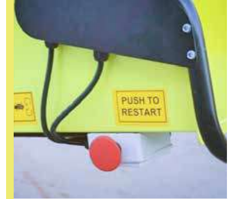
Emergency/ re-start buttons.
