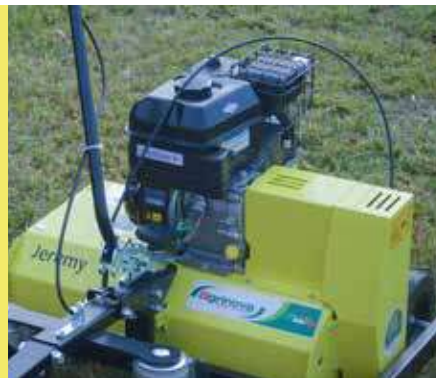
Central engine position for optimum weight balance.
