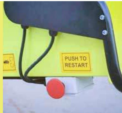
Emergency/ re-start buttons.
