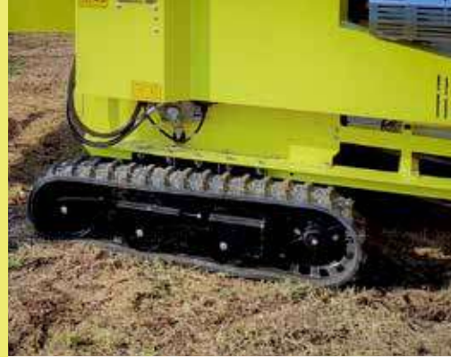
Great stability thanks to quality tracks produced in Italy . 1 mt track.
