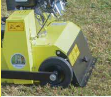
200 mm diameter solid rubber wheels with sheet metal rims.
